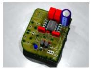
After spending days reading tutorials, message boards, shopping for parts, and then tweaking a cMoy on a breadboard, I spent more than eight hours constructing my first hand built cMoy on protoboard. It didn't work. I spent another eight hours assembling a second (and functional) cMoy, later realizing I had forgotten just one wire on each channel of the first amp. In all, it took over 25 hours to build the same amplifier many others before me had built over the previous eight years.
